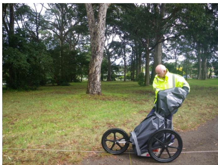
Figure 3: Survey area with scan in progress. Tapes were used to ensure that correct line separations and directions were achieved.
